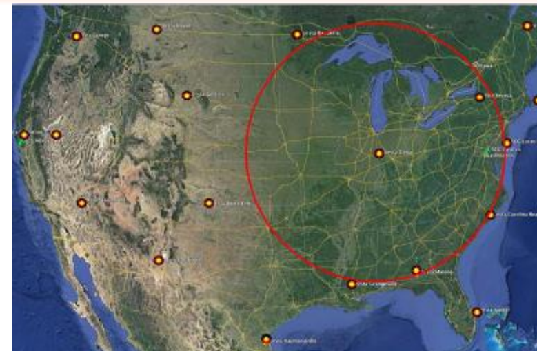
The 19 legacy US eLoran Towers: This circle represent the effective range of single tower
