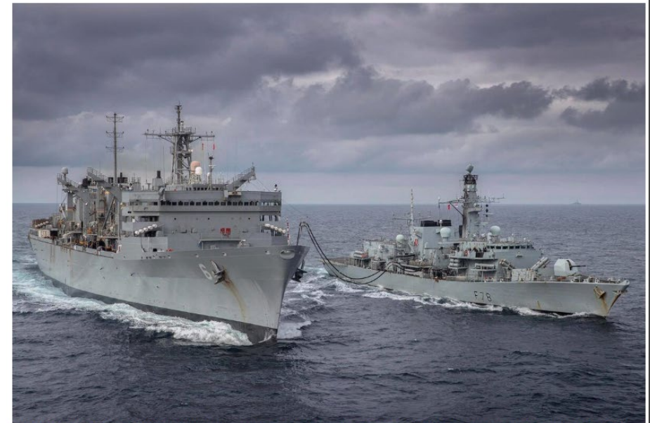
The Duke-class frigate HMS Kent (right) takes part in a replenishment-at-sea with Supply-class fast combat support ship USNS Supply (T-AOE-6) while on exercise with the U.S. Navy in the Arctic Circle. (Dan Rosenbaum/ HMS Kent)
