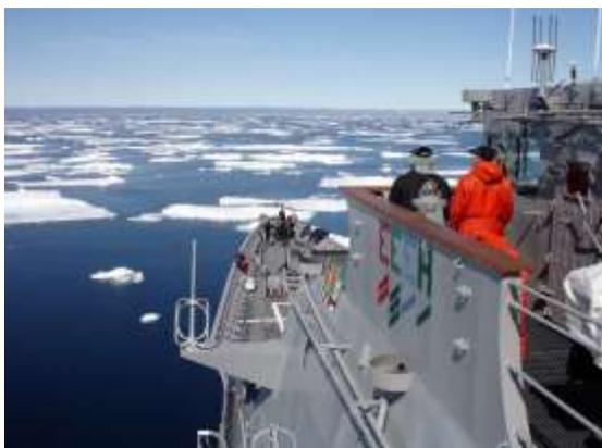
*Non ice-strengthened vessels working in ice covered waters and Sailors wearing Damage Control gear for cold weather protection*
